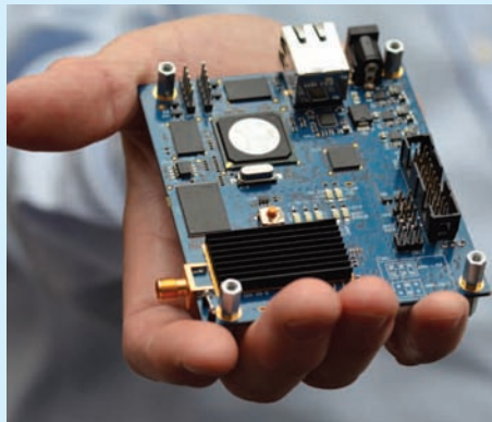
Sidewinder is one of the smallest commercially available 2G and 3G small cell platforms. The device has been developed by Cambridge Consultants to offer a low cost of entry for companies wishing to exploit a range of mobile communications standards
